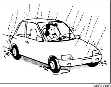
Under wet road conditions you should drive at a lower speed than on dry roads due to possible slippage of tires during braking. When driving on icy, snow-covered, or muddy roads, reduce your speed and avoid sudden acceleration, abrupt braking, or sharp steering movements.
